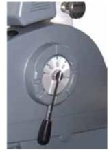
5 position lever adjusts the nip between the rollers while springs maintain even pressure during lamination.
