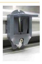
cutter permits simple cutoff as the laminated material exits the rear
